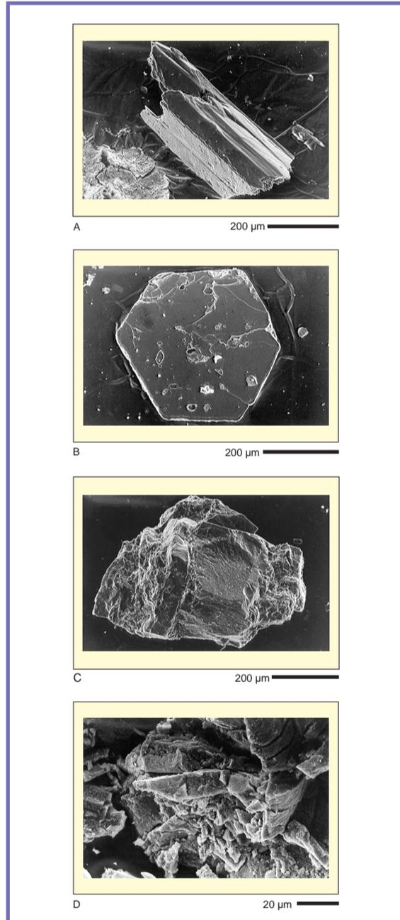
Figure 3 SEM photomicrographs of fine-grained heavy minerals found in the Ordovician sequence of Sama-Chaupi Uno. A. Prismatic grain of Ca-Pyroxene. B. Euhedral grain of biotite with pitch structures. C. Alternation of apatite layers and siliciclastic material. D. Chromite grains in concretions of Fe-oxides.
